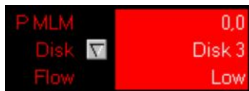
Fig. 3.12: Low – Pressure differential at the disk is too low
