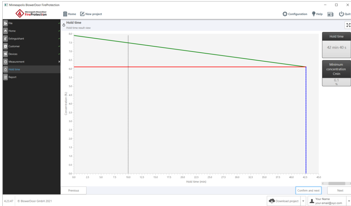
Fig. 6.47: Display of the hold time for extinguishants with the same density as air or force mixed
