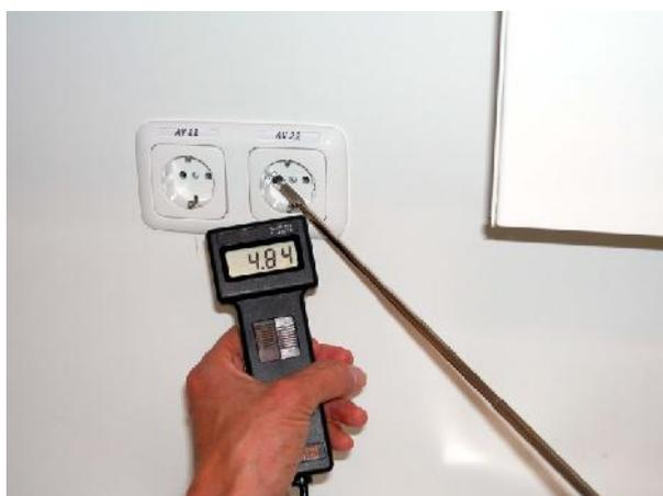
*Leakage detection during the BlowerDoor test*
