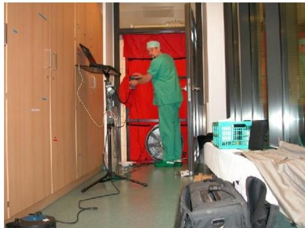
*Testing the airtightness with the measurement system Minneapolis BlowerDoor*
